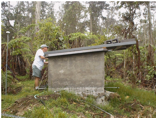
Figure 5. Instrument vaults. Six-inch concrete walls and steel lids ensure the equipment's survival in the case of a tree fall. Each vault is locked. Pipes for connecting the wind-noise reducing filters are connected to a summing manifold imbedded in the vault's foundation.
