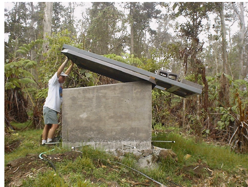
Figure 5. Instrument vaults. Six-inch concrete walls and steel lids ensure the equipment's survival in the case of a tree fall. Each vault is locked. Pipes for connecting the wind-noise reducing filters are connected to a summing manifold imbedded in the vault's foundation.
