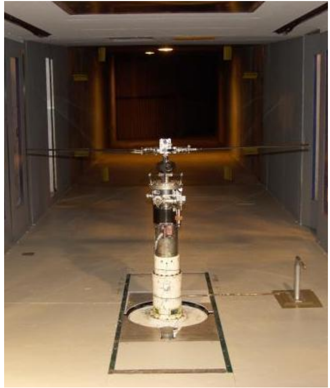
Fig. 1. Installation photo of US Army RWTS stand and teetering hub in 7- by 10-Foot Wind Tunnel.
