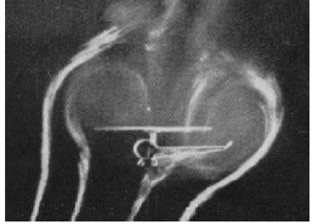
Figure 1. Smoke flow visualization of a rotor in vortex ring state (Drees, Ref. 20).
