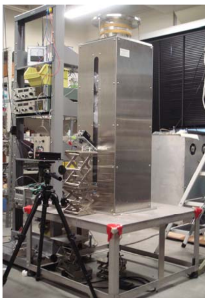
Fig. 4 YD-2. The plasma is produced in a vapor of liquid helium.
