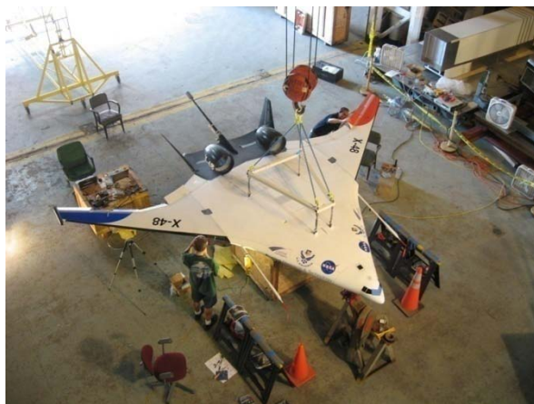
Figures 16 and 17. Boeing X48C Vertical Stabilizer Placement
