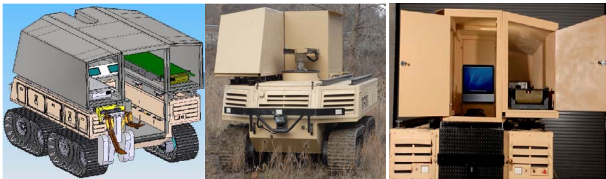
Figure 4. Tactical Amphibious Ground Support System – Common Experimental (TAGS-CX) with Patient Transport and Operator/Attendant Modules
