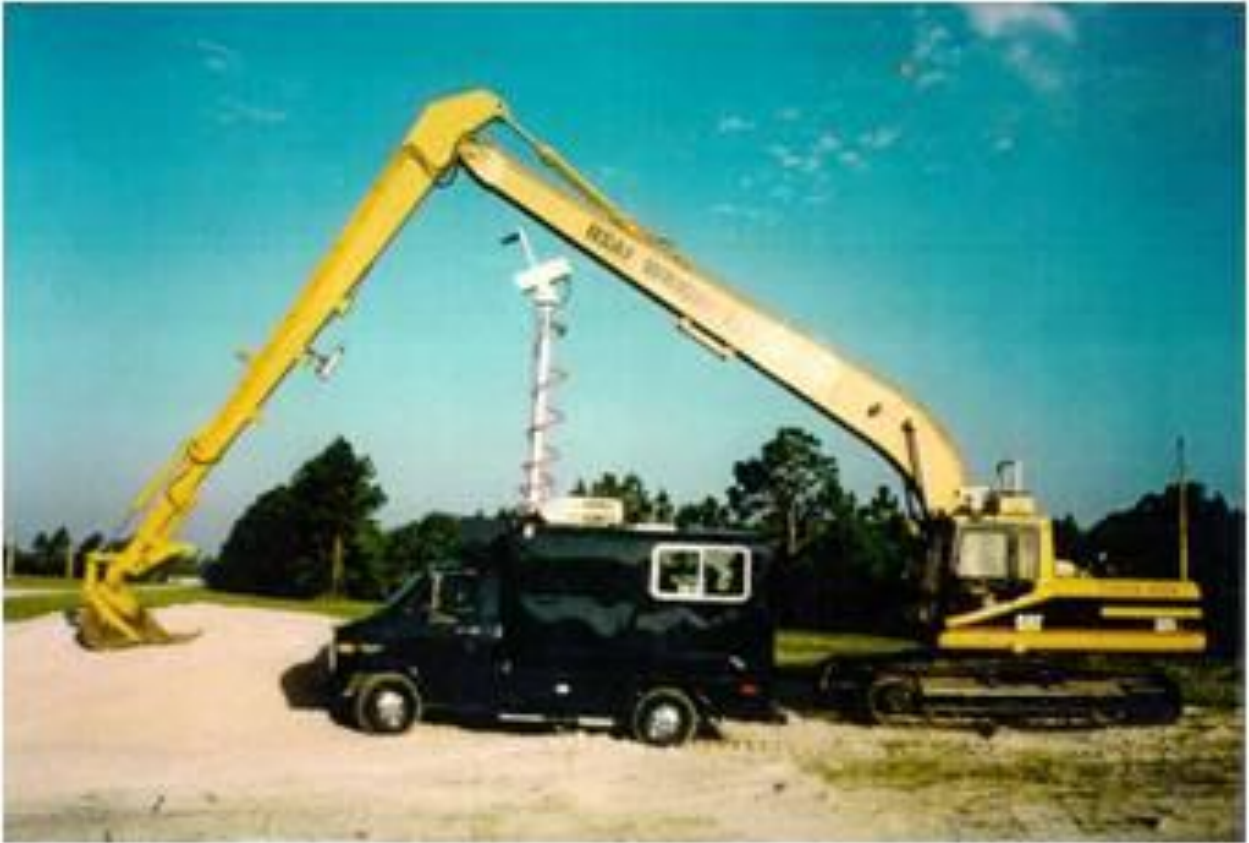
Figure 5: Mobile Command Center for Teleoperated Equipment
