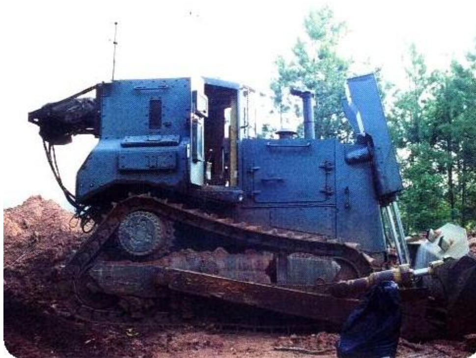
Figure 1: Armor Plated D8N Bulldozer with Blade
