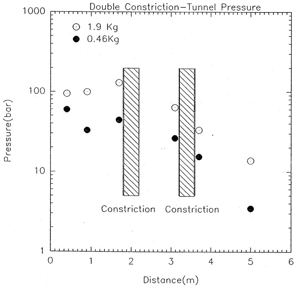
**Fig. 12. Pressure vs. Distance in the access tunnel for the double-constriction magazine.**
