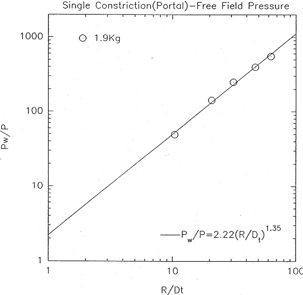
**Fig. 15. Scaled Pressure,  $P_w/P$  vs. Scaled distance,  $R/D_t$  in the free field for the portal-constriction magazine.**
