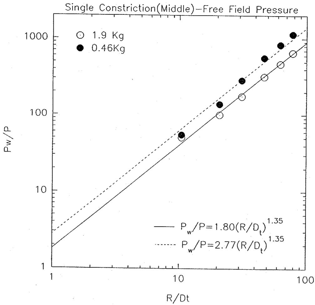
**Fig. 14. Scaled Pressure,  $P_w/P$  vs. Scaled distance,  $R/D_t$  in the free field for the middle-constriction magazine.**
