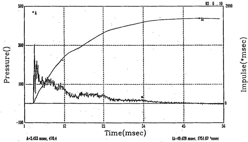
Fig. 7. Pressure-time histories in the access tunnel.
