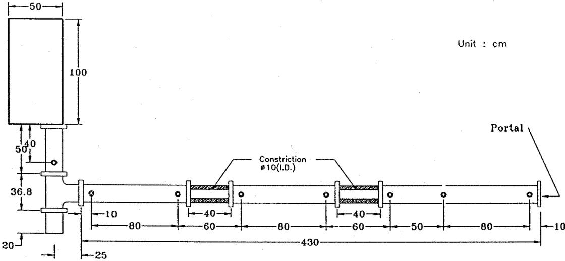
**Fig. 4. The double-constriction magazine.**
