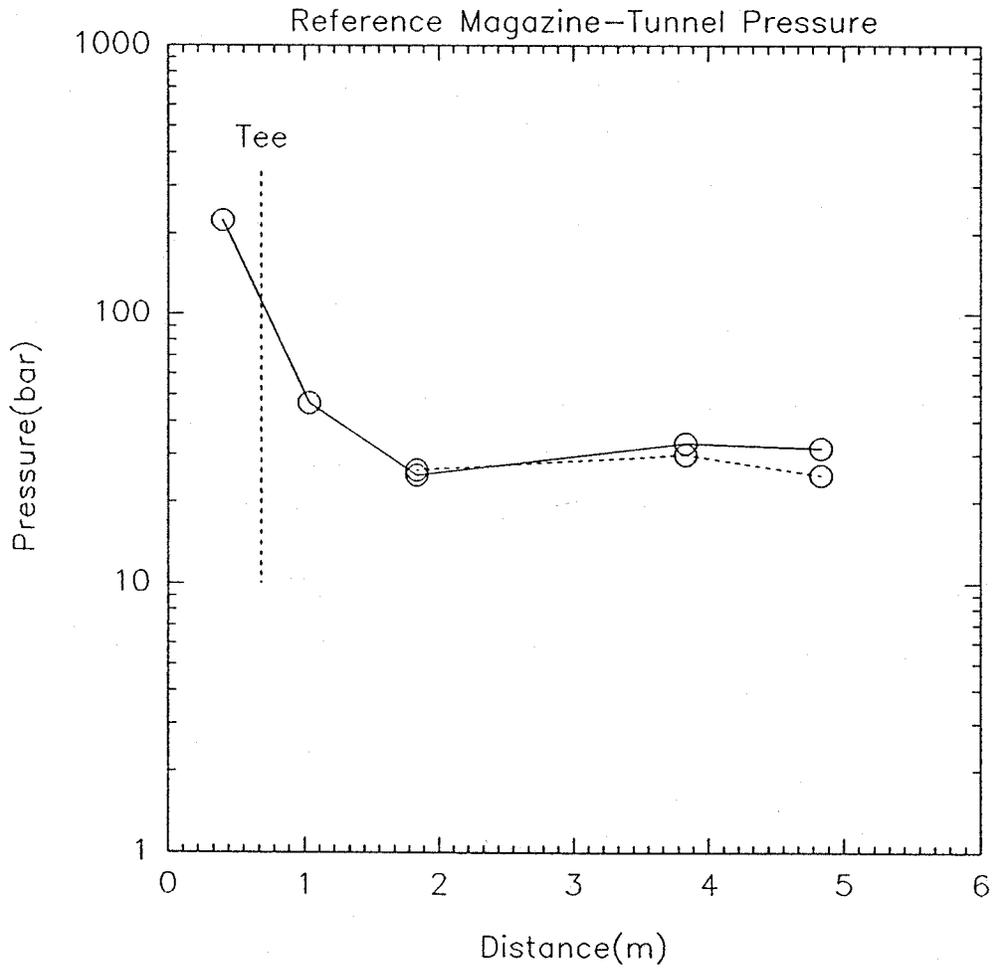
**Fig. 9. Pressure vs. Distance in the access tunnel for the reference magazine.**
