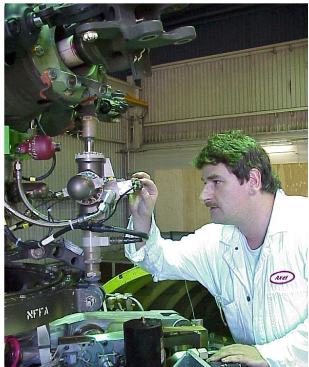
Fig. 3. IBC actuator installed in the rotor system.
