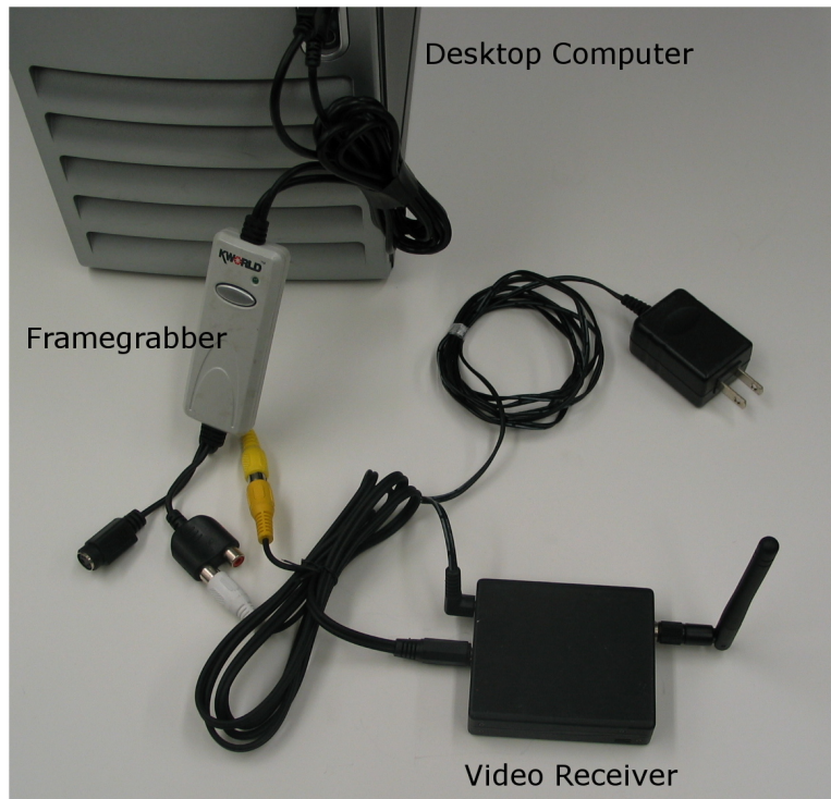
Figure 2.5: Video hardware used at the ground station to acquire video from the UAV and convert it to a digital signal for processing on the ground station computer.
