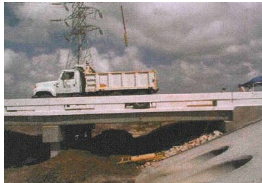
Figure 25. HS-20 test load of the TxDOT San Patricio County bridge.
