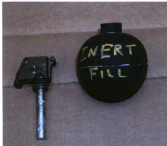
Figure 3 Modified M67 grenade w/inert M213 fuze
