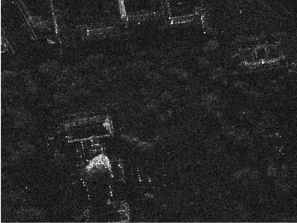
Figure 17. Ku-band SAR image with simulated \sigma_N = -20 dB.
