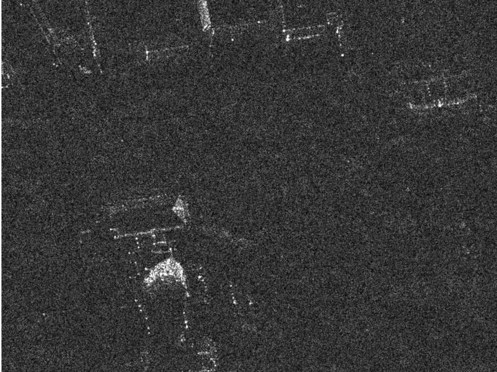
Figure 18. Ku-band SAR image with simulated \sigma_N = -15 dB.
