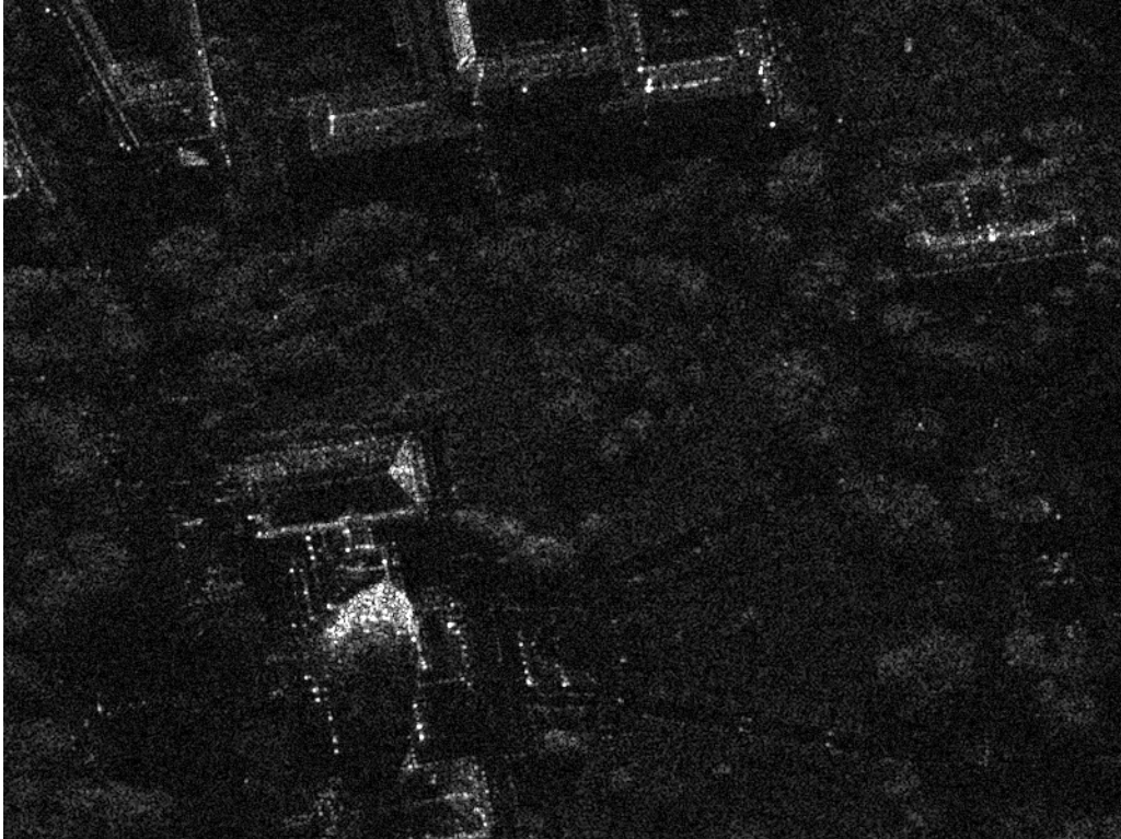
Figure 16. Ku-band SAR image with simulated \sigma_N = -25 dB.
