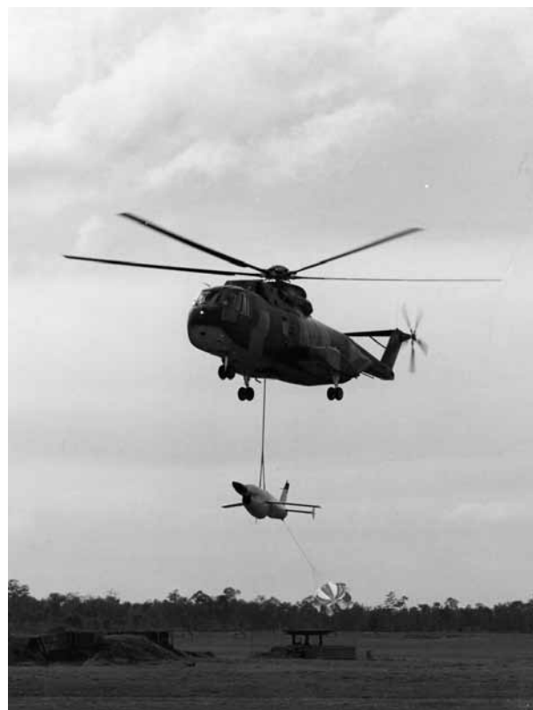
A CH-3 helicopter returns to home base after recovering an AGM-34 RPV.
