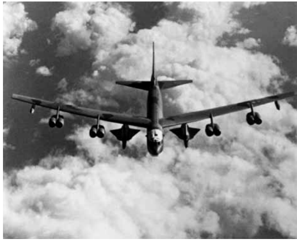
Two D-21 drones carried aloft by a B-52, which succeeded the A-12 aircraft as mothership.
