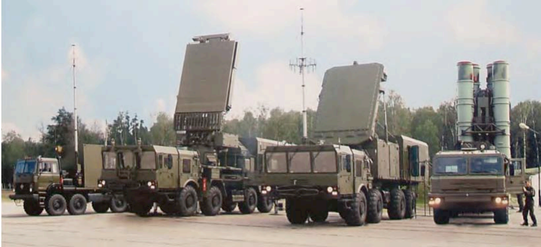
International sales of advanced IADS, such as the SA-21A shown at right with 92N2E engagement radar and 96L6E surveillance radar, could present potential anti-access/area-denial capabilities.
