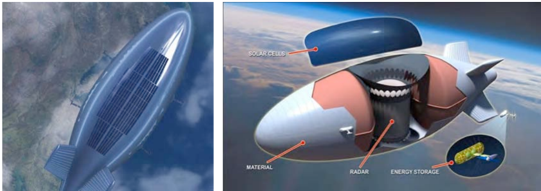
Figure 15. High-altitude long-endurance ISR airships can remain aloft for years, so that launch/ascent are decoupled from immediate demand and thus can be timed when winds are low. This allows exceptionally lightweight structures to be used that can enable extreme functionality.
