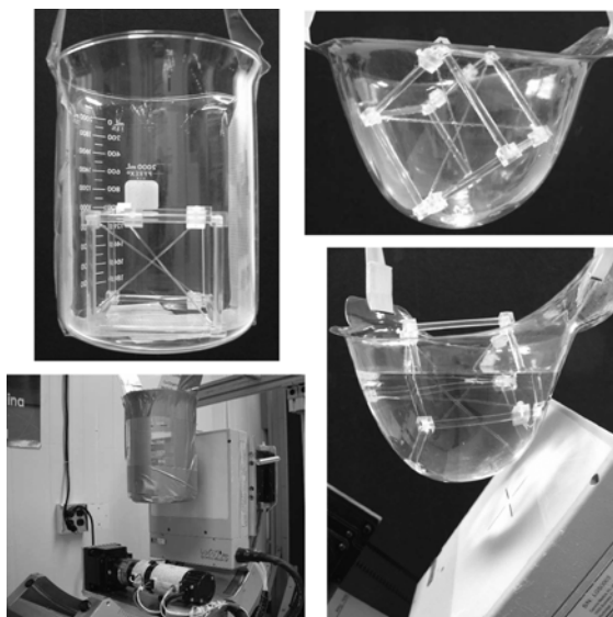
Fig. 3. Photographs of the MTF phantom contained inside (Left) the 2000 mL cylinder and (Right) 850 mL breast phantom shell. (Bottom) Phantom was immersed in the water to the extent possible to quantify the effect of different object shapes along with various acquisition trajectories on the MTF, and (Top) is also shown in the phantoms without water present.
