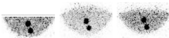
Fig. 9. MIP images of reconstructed data set to a global maximum containing acrylic (top) and thin-walled (bottom) radioactive lesion phantoms.
