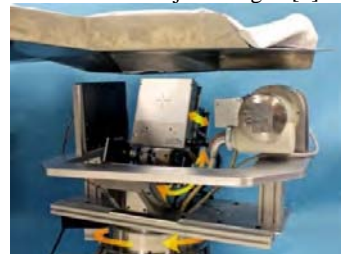
Fig. 1. Hybrid SPECT-CT breast imaging device. Orange and yellow arrows indicate the directions of movement of the SPECT camera (center).
