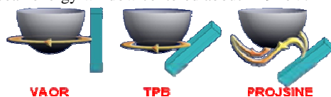
Fig. 5. 3D trajectories (yellow path) of the gamma camera (blue box) used to acquire data.
