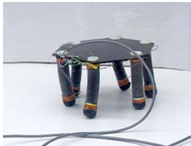
Figure 6: MERbot, a robot using a 2-DOF spring roll as each of its six legs.
