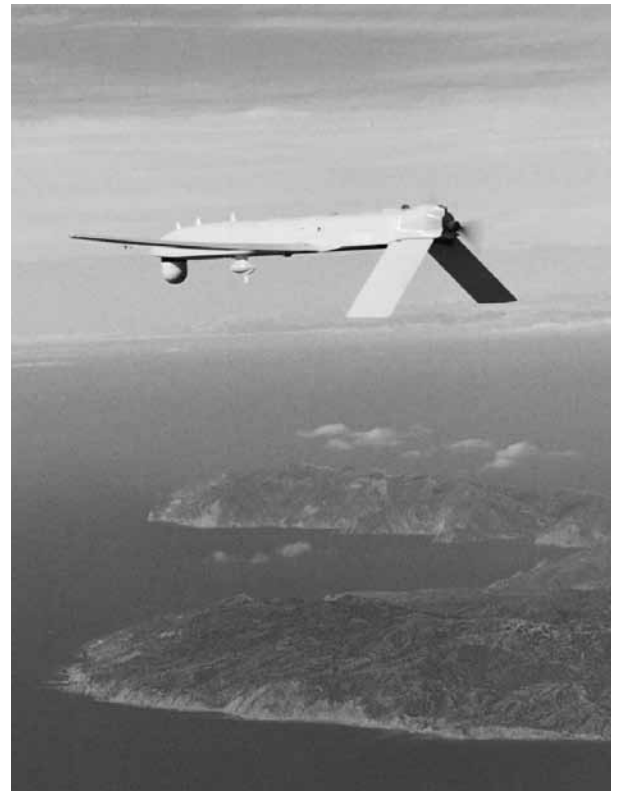
A version of the General Atomics Aeronautical Systems Gnat 750 (originally developed by Abraham Karem) known as Tier I in OSD's RPV acquisition strategy of the early 1990s and employed by the CIA.
