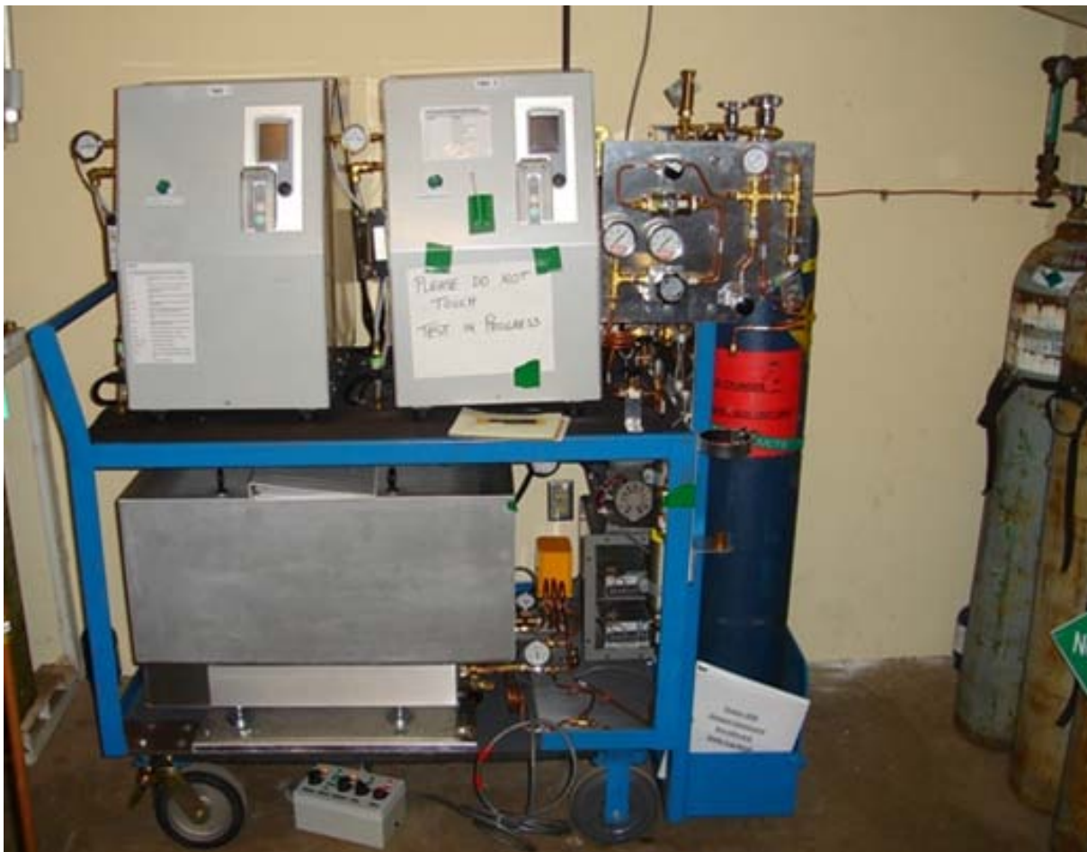
Photograph #1. SEOS breadboard installed at OC-ALC maintenance facility.
