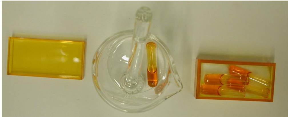
Figure 2-2. Neogen ® Agri-Screen Oxidation Materials. Shows a top view of the bromine capsule container lid, bromine capsules, 100 ml beaker and glass rod provided by Agri-Screen.
