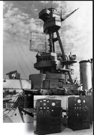
In 1939, the battleship USS New York (BB-34) receives the United States' first radar, the XAF, developed by NRL.
