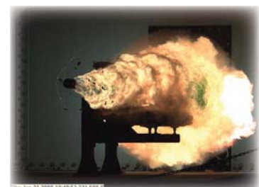
World record is set for an electromagnetic railgun fire at 10.64 mega joules with a muzzle velocity of 2,520 meters per second at the Naval Surface Warfare Center, Dahlgren, VA January 31 2008
