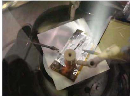
Figure 6. Test fixture used in the variable temperature LCR measurements on metallized polymer films
