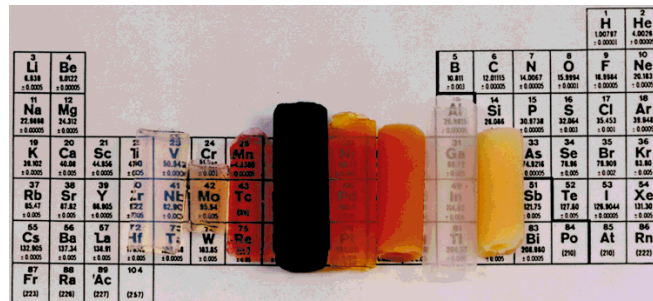
Fig. 3. Silica-based composite aerogels (from left to right): pure silica aerogel [overlying Ti-V/Zr-Nb/Hf-Ta in the periodic table]; colloidal Pt-silica composite aerogel (2 nm Pt sol); colloidal Au-silica composite aerogel (30 nm Au sol); carbon black-silica aerogel (Vulcan carbon black, XC-72); poly(methylmethacrylate)-silica composite aerogel (polymer M_w \sim 15,000 , sieved to <44 \mu\text{m} ); \text{Fe}^{\text{I}}(\text{bpy})_3\text{NaY} zeolite-silica composite aerogel (0.1–1 \mu\text{m} type Y zeolite crystallites modified with iron(i)tris-bipyridine); titania (aerogel)-silica composite aerogel ( \mu\text{m} -sized particulates composed of ~15 nm \text{TiO}_2 aerogel domains); and titania-silica composite aerogel (20–40 nm Degussa P-25 \text{TiO}_2 ). All samples shown are ~1 cm diameter monoliths of varying lengths.
