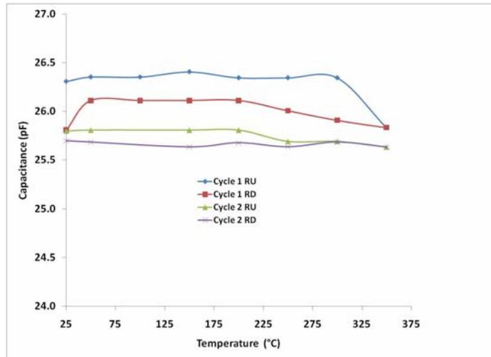
**Figure 11.** Film capacitance (10 kHz) over two complete thermal cycles up to 350°C for the FDPAE polymer
