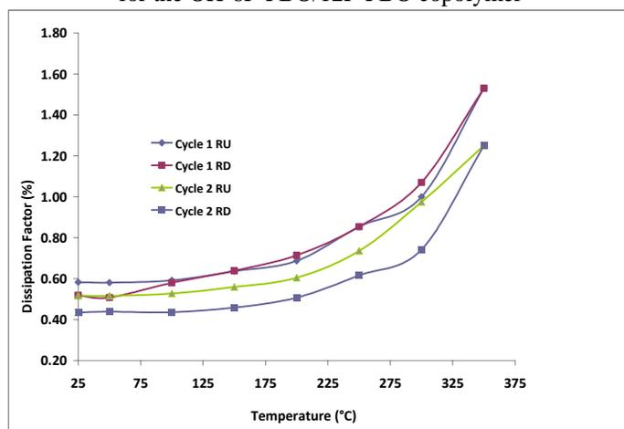
**Figure 8.** Film Dissipation Factor (10 kHz) measured over two complete thermal cycles up to 350°C for the OH-6F-PBO/12F-PBO copolymer
