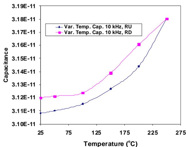
**Figure 6.** Capacitance in Farads (measured at 10 kHz frequency) as a function of thermal cycling for the OH-6F-PBO/12F-PBO copolymer film (RU and RD refer to ramp up and ramp down during one complete thermal cycle).
