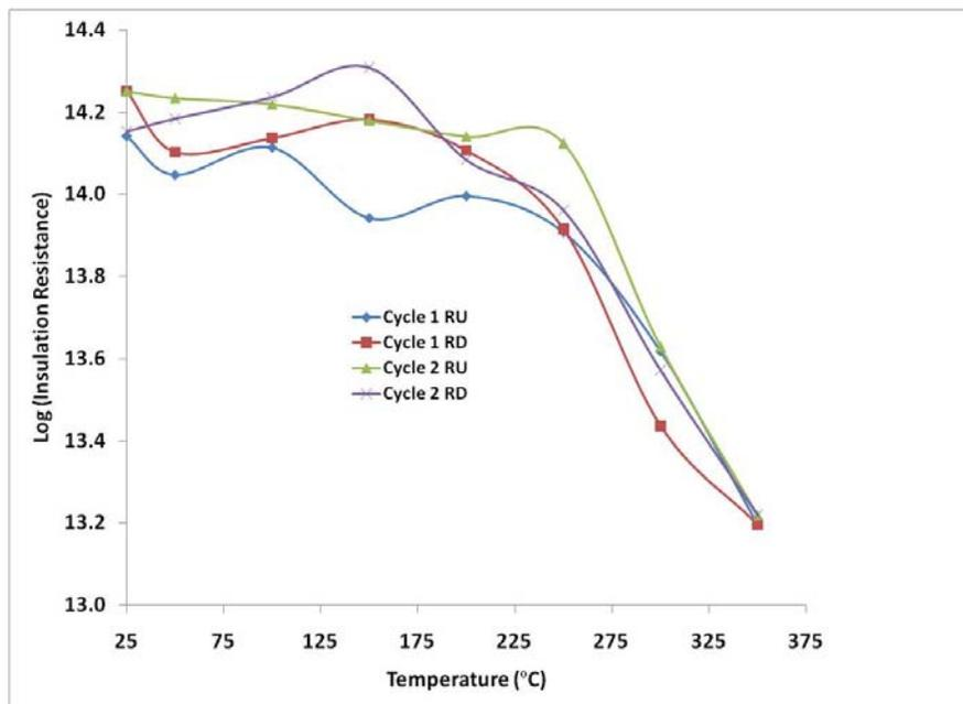
**Figure 13.** Insulation resistance of a metalized FDAPE film as a function of thermal cycling in the RT-350°C range
