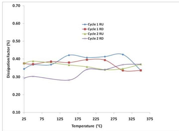
**Figure 12.** Film dissipation factor (10 kHz) over two thermal cycles up to 350°C for the FDPAE polymer
