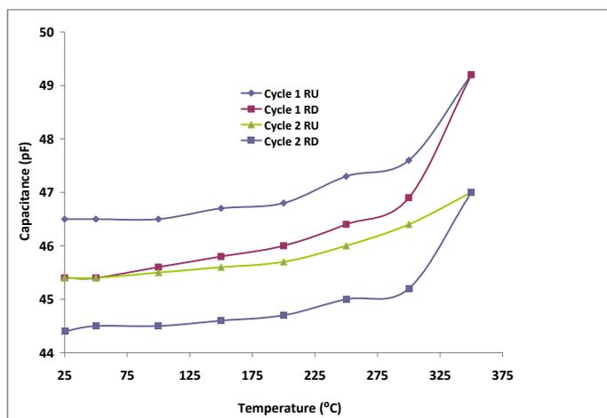
**Figure 7.** Film capacitance (10 kHz) over two complete thermal cycles up to 350°C for the OH-6F-PBO/12F-PBO copolymer
