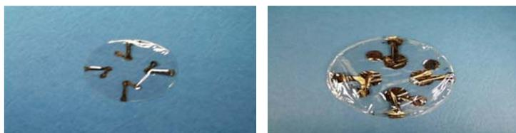
**Figure 3.** Single film device structures of FDAPE with circular Al contacts
