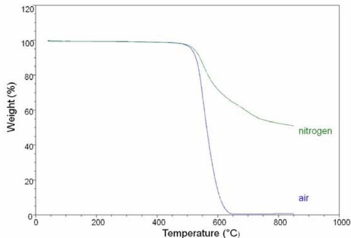
**Figure 2.** TGA traces of OH-6F-PBO/12F- PBO copolymer
