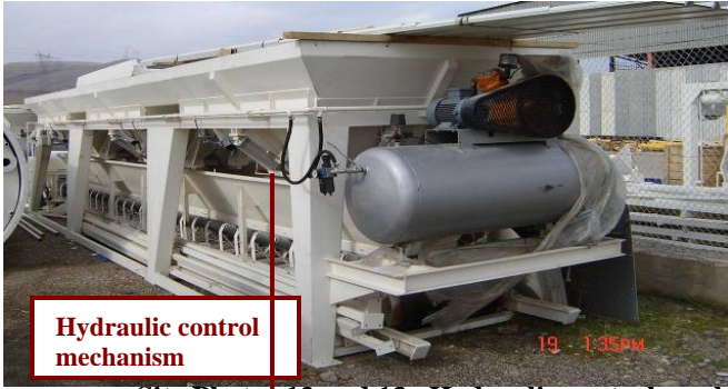
Site Photos 12 and 13. Hydraulic control mechanism and aggregate handling components with for the delivered 30-m 3 /hour concrete-mixing plant.
