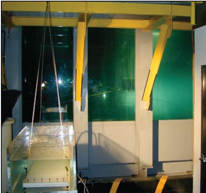
FIGURE 1 Exterior view of the Salt Water Tank, with a small bubbler test tank on the left. The main tank measures 6 m x 6 m x 4 m deep, although typical water depth is 3 m. The interior of the tank has 50 precision-controlled air-flow ports to allow for various air injection mechanisms to be arranged for each experiment. Barely visible at the far left is the salt mixing tank used to mix salt into the main tank to any desired level of salinity. Visible through the Plexiglas windows of the large tank is an ITC2010 acoustic source, used for much of the experimental data below 10 kHz.
