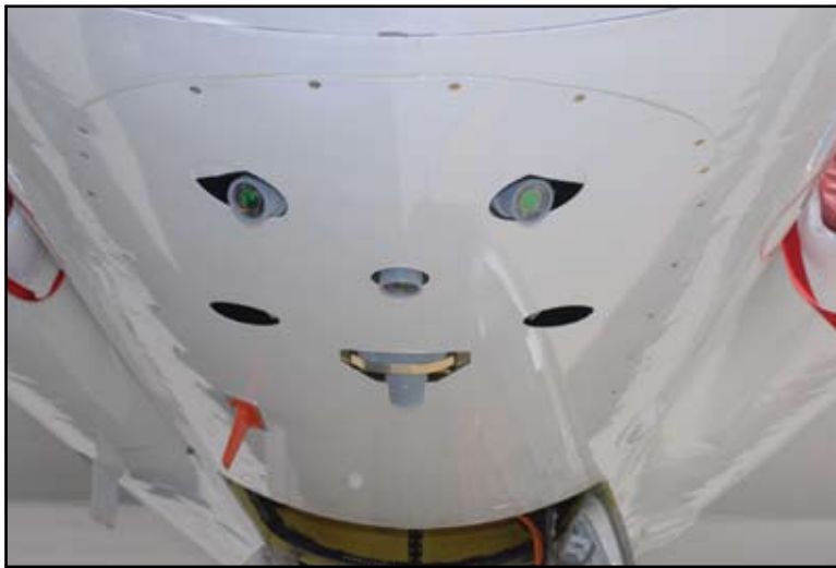
FIGURE 2 CHLOE sensors mounted in lower ER-2 Q-bay hatch.
