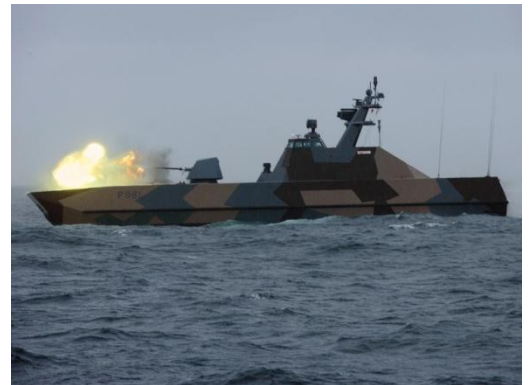
Figure 1: The Norwegian Skjold-class Full load: 270 t Length: 47.5 m (156 feet) Beam: 13.5 m (44 feet) Draft on cushion: 0.9 m (3 feet) Draft off cushion: 2.3 m (7.5 feet) Maximum speed: 55 knots +
