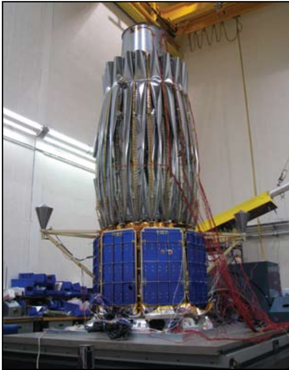
FIGURE 6 Photograph of the fully configured COMMx payload with the integrated TCS.
