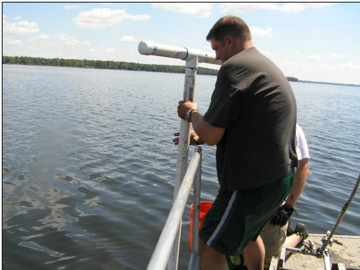
Figure 3. PVC-core sampler being deployed.
