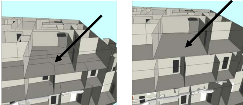
Figure 6-10 Left: Decks not separated, floor lines are shown; Right: Decks separated, no floor lines are shown
