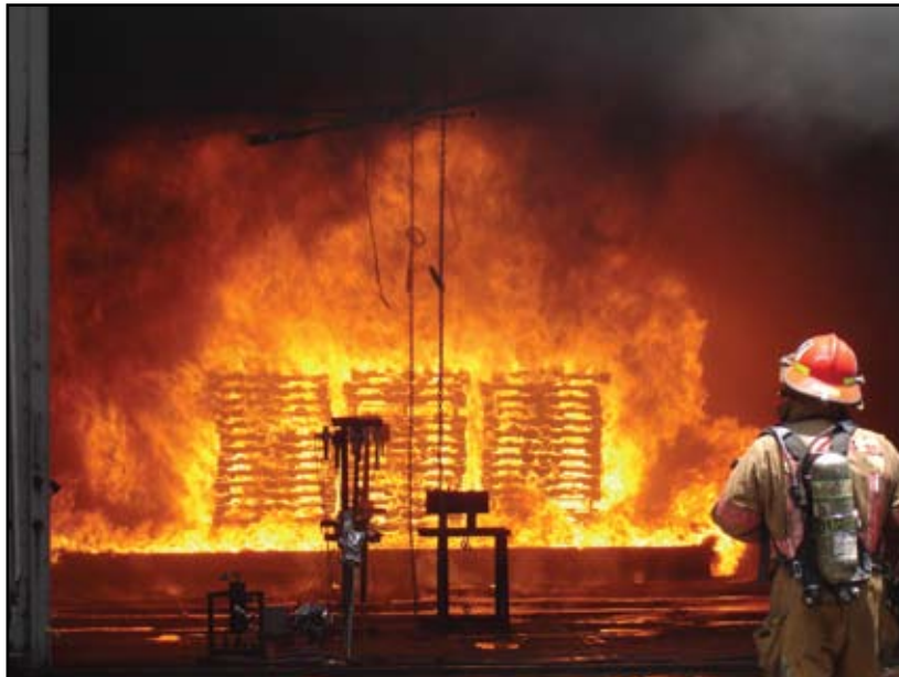
FIGURE 4 Quadruple 98 MW test fire prior to HotFoam activation.
