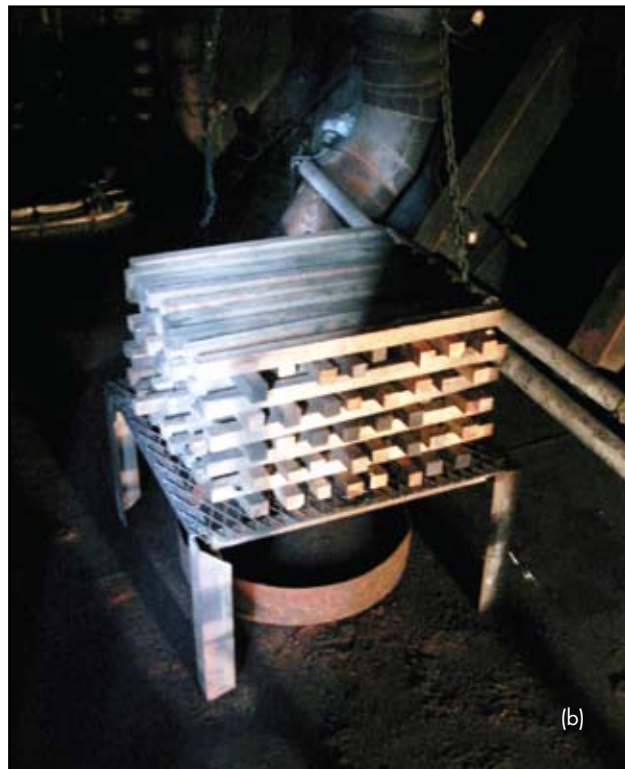
FIGURE 3 (a) Well Deck Mixed Class A and Class B Fuel Package. (b) Class A fuel package for the adjacent space fire.
