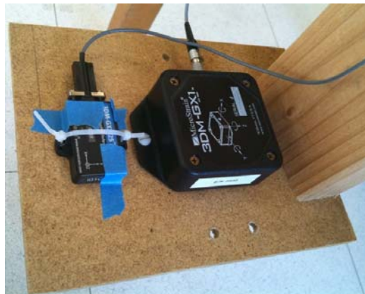
Figure 18. Sensors on Mounting Board, Attached to Pendulum.
