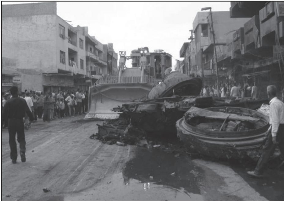
Figure 149. Engineers clear the streets with a D9 armored bulldozer
