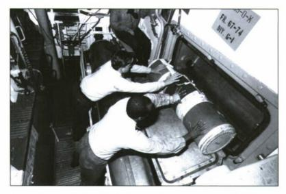
During the investigation into the *Iowa* explosion, a gun crew at Dahlgren demonstrates a proper bag charge ram by loading three powder bags into a 16-inch gun. (Dahlgren Historic Photograph Collection)
