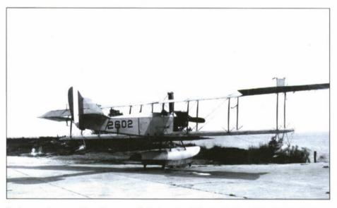
Early experiments with radio-controlled aircraft culminated in the 15 September 1924 flight of this N-9 seaplane, the first aircraft ever launched, maneuvered, and then landed intact under full remote control. (Dahlgren Historic Photograph Collection)
