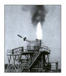
An 800-pound, 12.75-inch rocket leaves the muzzle of Weapon "Able" at Dahlgren's rocket battery. While working with Weapon Able in 1950, Dr. Charles J. Cohen developed the world's first operational six-degrees-of-freedom trajectory simulation, making possible the development of guided ballistic missiles. (Dahlgren Historic Photograph Collection)
