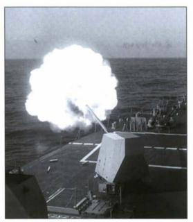
The high energy Mk 45 Mod 4 Gun Mount, installed on the USS Winston S. Churchill (DDG-81) with an all-digital fiber-optic interface to the onboard Mk 160 Gun Computer System (GCS), fires an ERGM slug to test the impact of 18 megajoule shots on the warship's structure. (Dahlgren Public Affairs Office)
