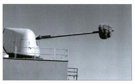
A Mk 45, 5-inch, 62-caliber gun fires down range, with the projectile just exiting the barrel. (Dahlgren Public Affairs Office)
