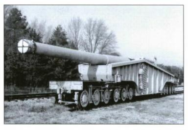
This 14-inch naval railroad gun was one of eight built for service on the Western Front in WWI. Five saw combat, but the war ended before this one ever fired a shot at the Germans. After returning to the United States, it became a terminal ballistics test bed at Dahlgren. BUORD's need to safely test such long-range guns led to Dahlgren's establishment. (Naval Historical Center)
