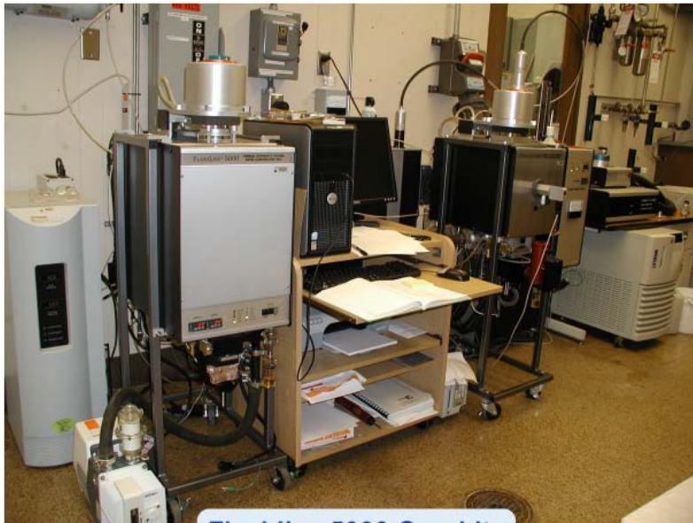
Flashline 5000 Graphite: 25 to 2500 °C @ inert gas
