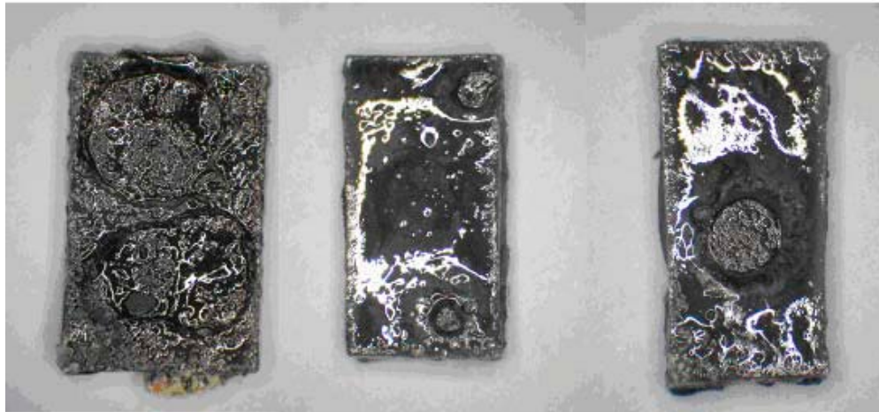
Fig. 3.65. Top surface view for USS 43 composite samples after oxidation.
