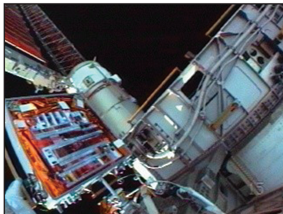
FIGURE 3 Thin-Film Materials Experiment on MISSE-5. The photograph was taken by Astronaut Soichi Noguchi's helmet camera while he was deploying MISSE-5.
