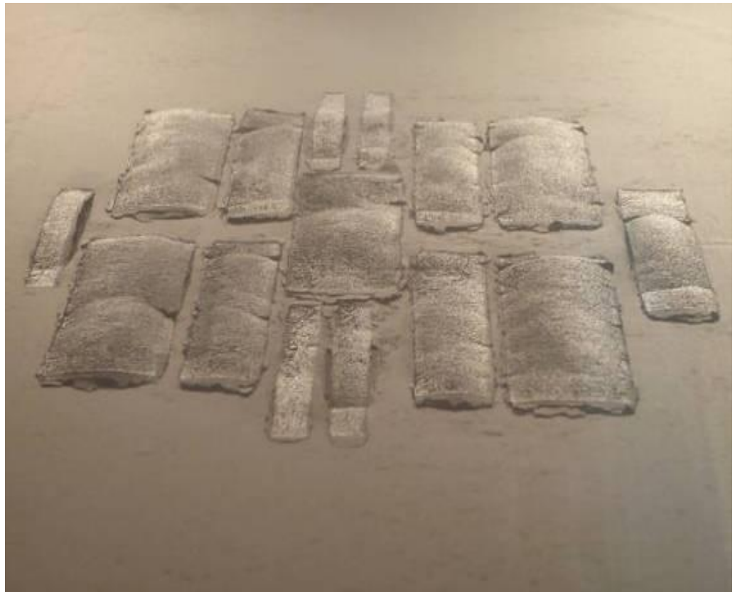
Figure 6 Warping of the 2 nd layer after laser scanning
