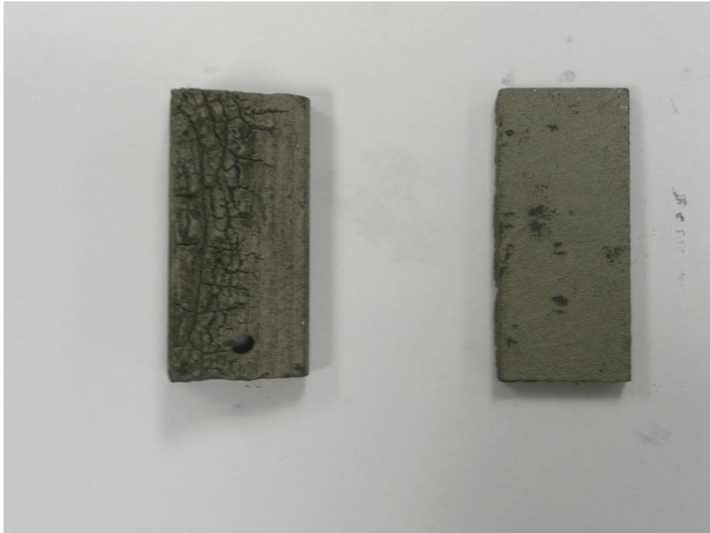
Figure 7 A fuel injector strut and a sacrificial plate built in RUN 5
