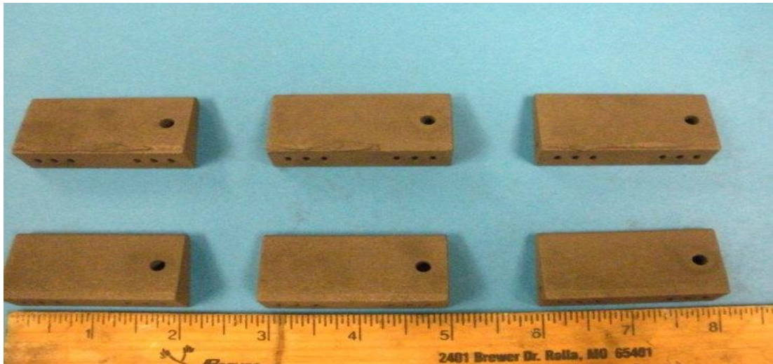
Figure 10 Green injector parts fabricated with separation of 5 (top) and 6 (bottom) layers
