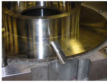
(a) U720 forging being machined (b) Predicted axial distortion (c) Measured distortion
