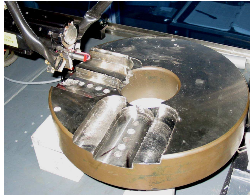
Figure 18. Machining of slots during measurement of residual stresses.
