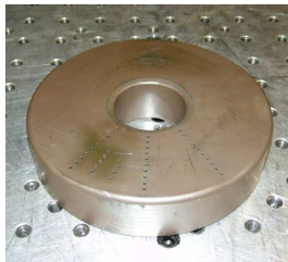
(a) U720 disk (b) Measurement Holes (c) Measured distortion (d) Predicted distortion
