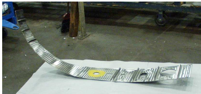
Figure 5. Distorted airframe component. This component was machined flat. The material stress and machining induced stress are causing it to distort.
