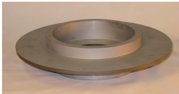
Figure 22. Forging after all four quadrants have been machined.
