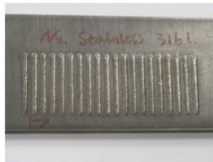
b. Nitrogen shield gas sample
