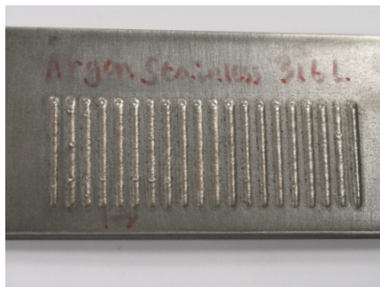
a. Argon shield gas sample
