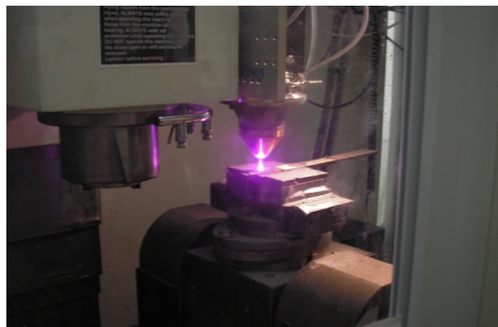
Fig. 1: Laser Aided Manufacturing Process deposition system
