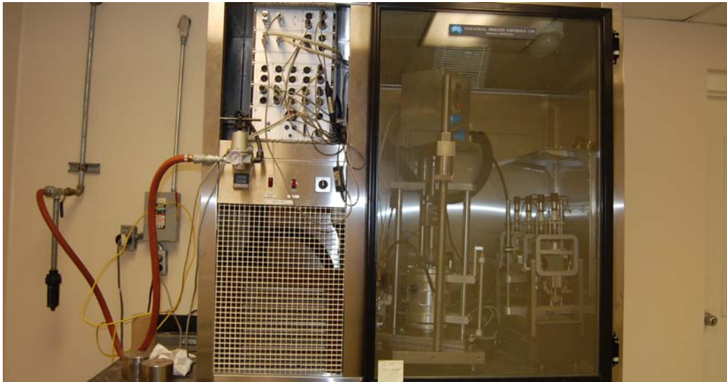
Figure 2. IPC universal testing machine (UTM 25) and temperature chamber used for static and dynamic creep tests.
