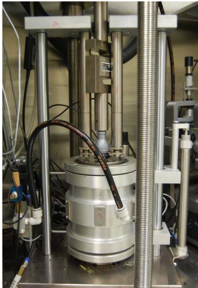
Figure 3. Test setup for confined creep tests.
