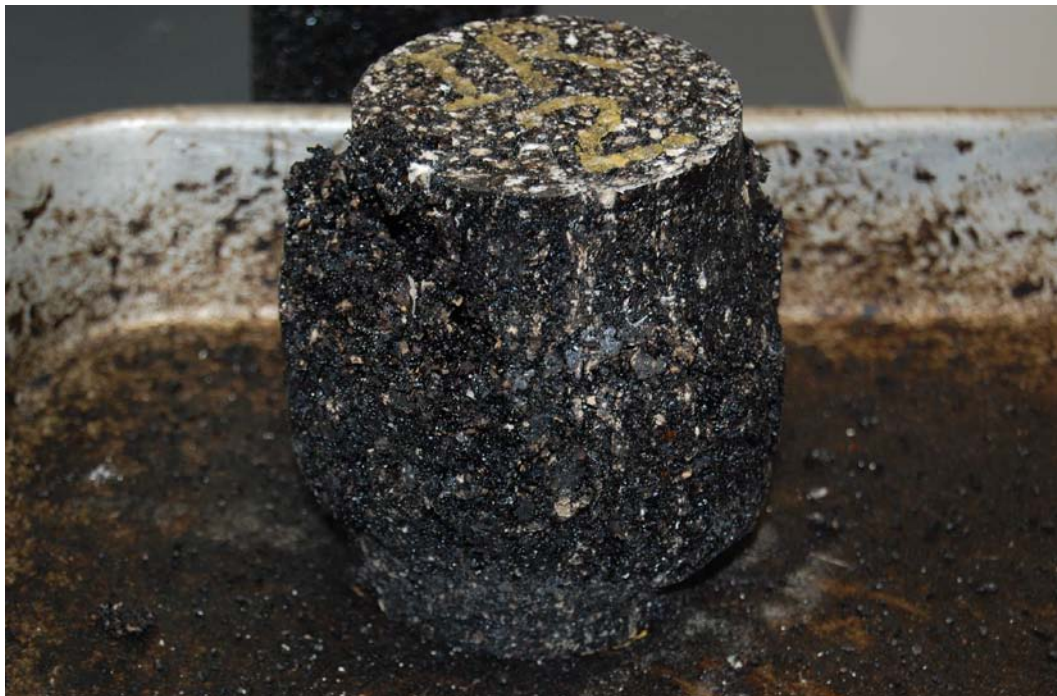
Figure 7. IRR sample after static creep test.
