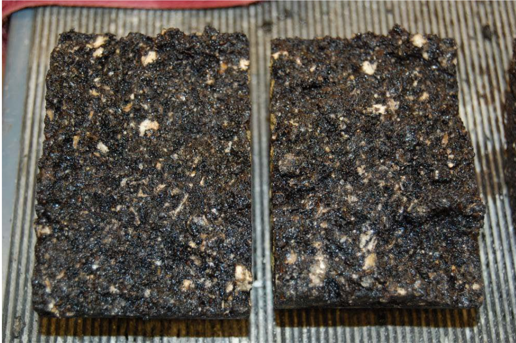
Figure 17. Broken aggregate on an EZ-Street sample.
