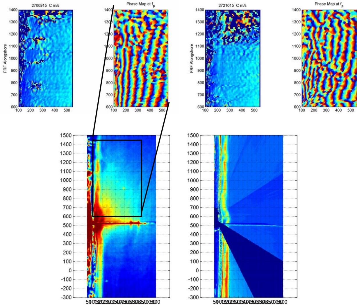
**Figure 3.** Upper panels are radar-derived phase speeds (C) and phase maps at the peak frequency ( $f_p$ ) from two days at Duck. Lower panels are (left) radar time exposure and (right) video time exposure from one day at Duck. Black square on lower left panel indicates the boundaries of the minigrid over which phase maps were calculated.
