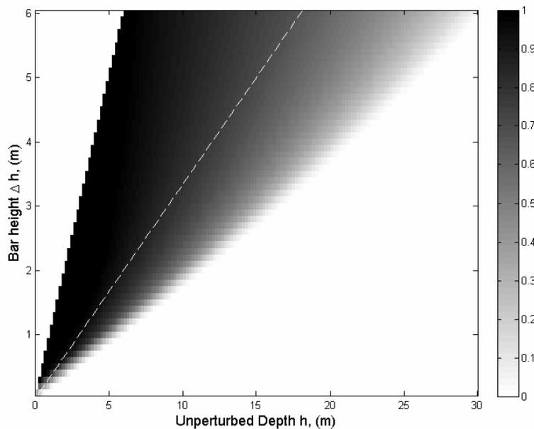
**Figure 1. Fraction of wave conditions in the range  $3 < T < 16$  sec,  $0.1 < H < 3.0$  m capable of detecting a sand bar (using nonlinear phase speed depth inversions). Dashed white line indicates typical bar height at each depth.**
