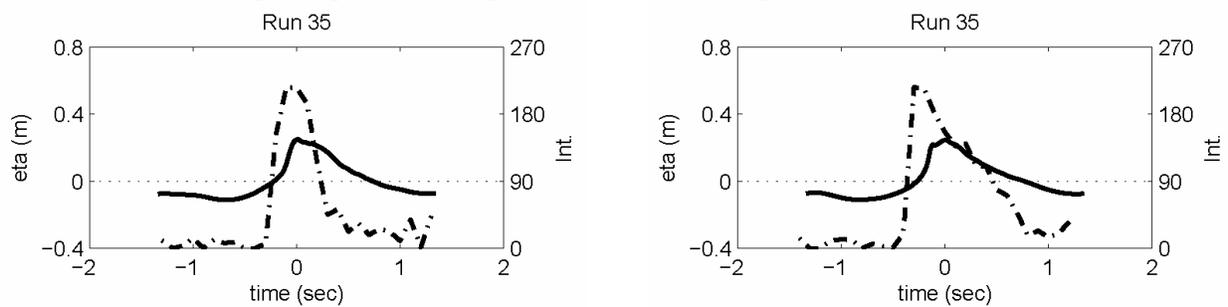
**Figure 2. Relationship between the phase-averaged water surface elevation (solid lines) and associated video intensity signals (dashed lines) for breaking waves. Results demonstrate the location of the intensity peak with respect to the wave crest.**
