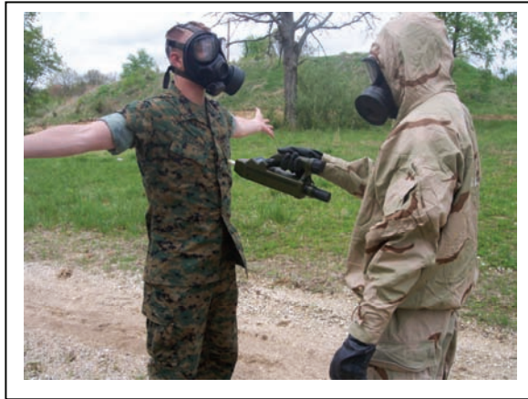
Figure V-8. Checking for Contamination
