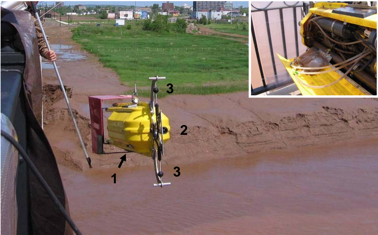
Figure 1: Profiling package deployed in the Petitcodiac River to observe the behaviour of fluid mud in a sheared flow. Instruments mounted on the package include 1) D&A optical backscatterance sensor and sample port for pumped samples (see inset), 2) Ocean Sensors CTD and 3) Marsh McBirney electromagnetic current meters.
