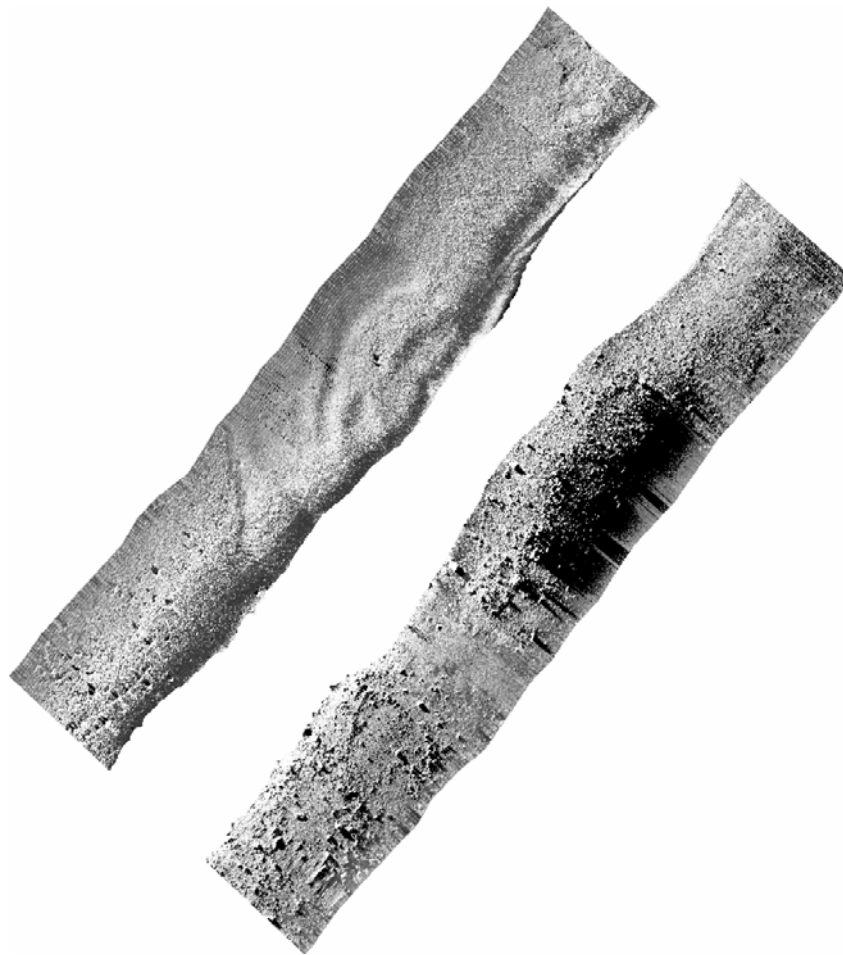
Figure 1. Top - Raw REMUS sidescan file. A strip of backscatter from the seafloor that shows much variation in intensity along track from ping to ping. Bottom - Processed data is geo-referenced and has been corrected for along track intensity variations.
