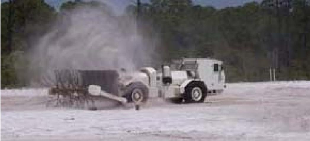
**Figure 1. Hydraema 910 Mine Area Clearance Vehicle**
