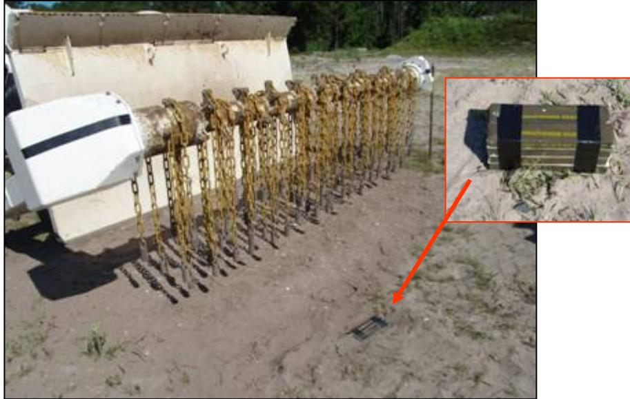
**Figure 4. Pre-test: 10-lb C-4 Charge**
