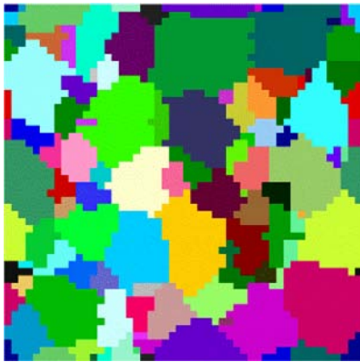
Figure 1 2-D section of a microstructure generated using the ellipsoid packing algorithm with a bi-modal grain size distribution.
