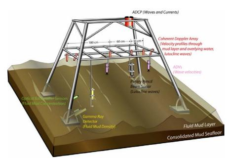
New sonars are being tested for use on the quadrapod to be deployed during the field experiment.
