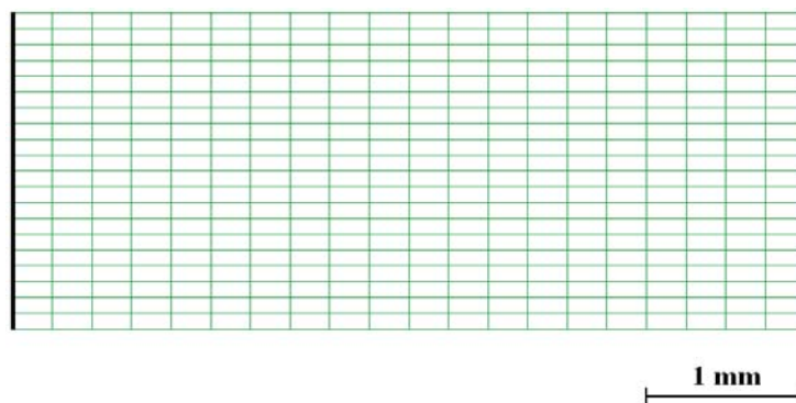
Figure 5: Axi-symmetric FEM model of a single free PZT element with a 20 \times 20 mesh
